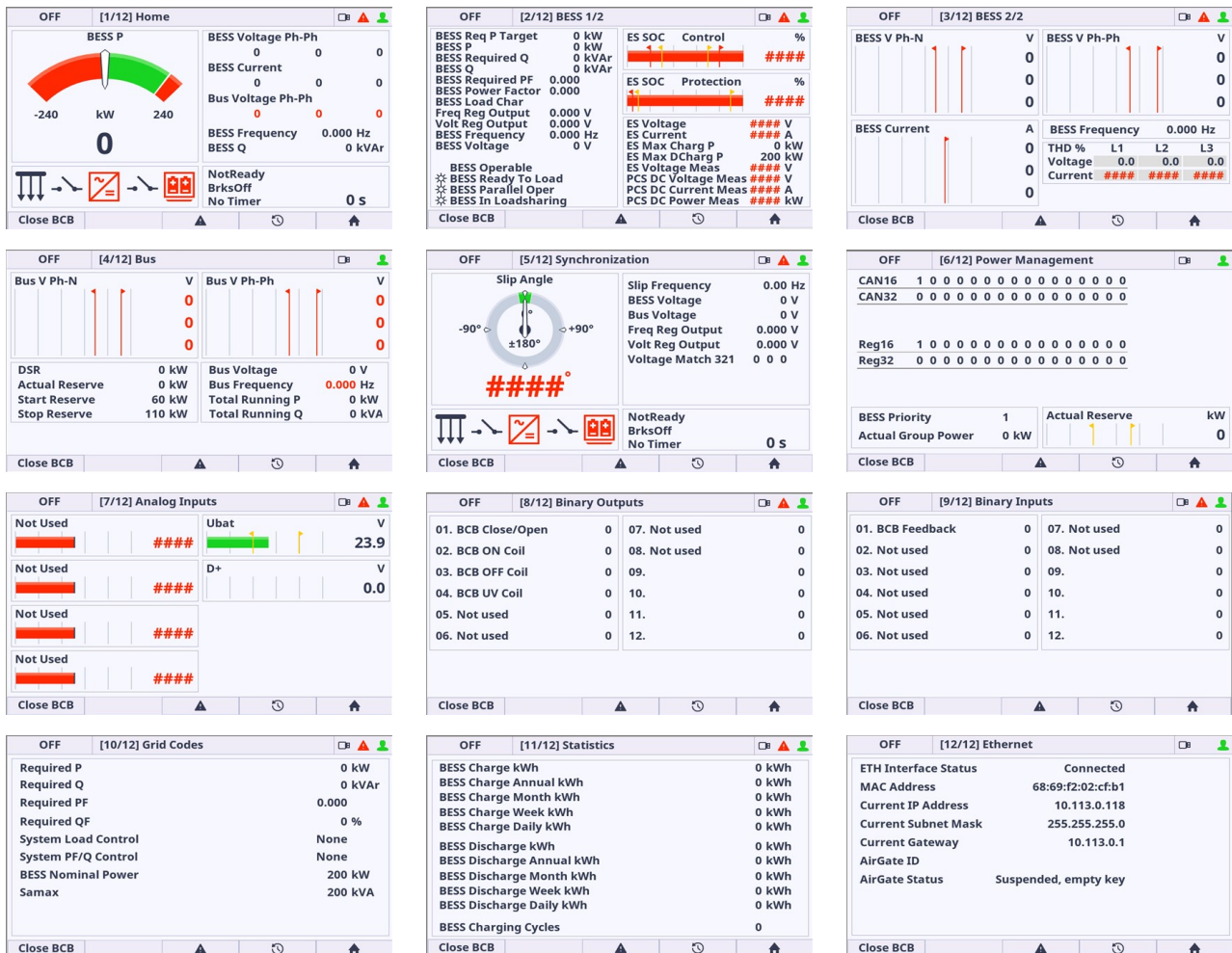
Image 5.16 : IntelliNeo 530 BESS metering screens overview
