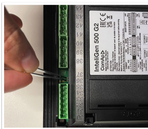
Image 5.73 Location of the DIP switch for Configuration override
