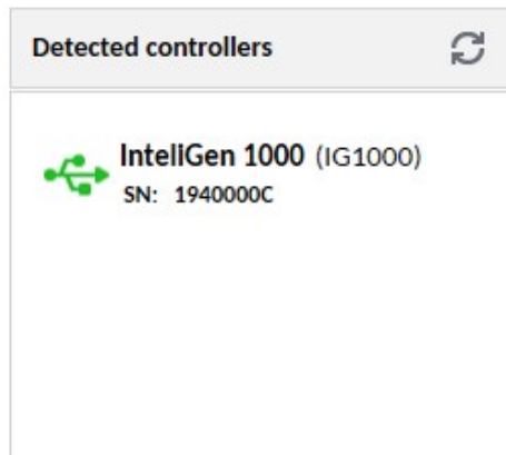
Image 5.48 Second screen of IntelConfig - Select your controller from list of Detected controllers.
