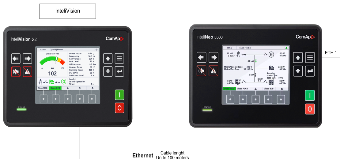
Image 4.44 Connection of IntelliVision display to IntelliNeo 5500
