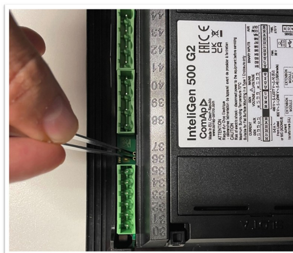
Image 6.12 Location of the DIP switch for Configuration override
