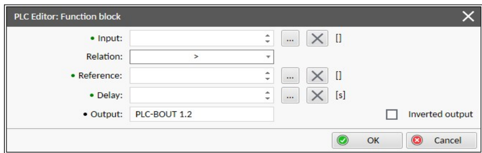
Image 21.52 Configuration of Comp Delay block
