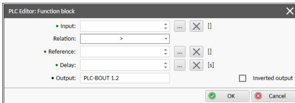
Image 15.7 Configuration of Comp Delay block
